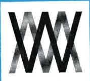
This is how the image of the filament will appear when the mirror is correctly adjusted.
