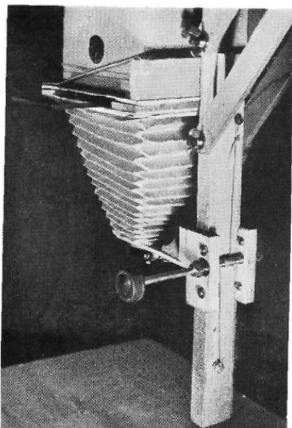
Turning the knob winds the lens smoothly up and down. Another popular focusing device for home-made enlargers consists of two tins or cardboard tubes sliding inside one another. Whatever method is employed the movement must be smooth, no part of the tube or bellows must obstruct the light from the negative and, most important of all, the lens must be exactly under the centre of the negative and exactly parallel to it at all times.
