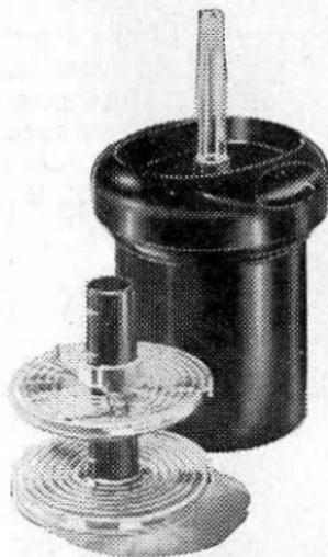
You have seen how easy it is to make your own prints, developing films is just as simple with the new Johnson Polly-Min Tank shown here. You can develop your size 20, 127 or 35 mm. films in less than an hour. The film is loaded into the spiral film holder in darkness, the lid is replaced and then all the developing, fixing and washing can be carried out in daylight. The Polly-Min Tank is almost unbreakable, holds only 10½ oz. of developing solution and is very reasonable in price.
